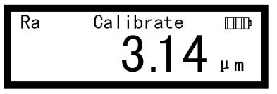
Put the instrument in the scribed line area. Sensor taxiing direction perpendicular to the scribed line of texture direction. Press the Start Key to exit the status of Calibration.
