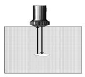
Fig. 1.1 Basic working principle for ultrasonic detection
